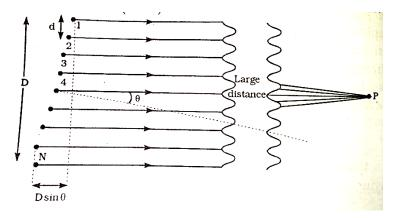
Consider the interference patterns produced due to the superposition of N vibrations of same period, amplitude and phase varying in in arithmetic progression.
