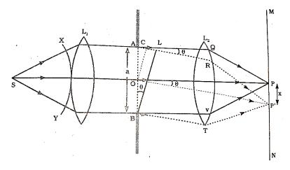
Consider a Source of light S produces divergent beam of light of wavelength  $\lambda$ . Those all ray are rendered to parallel beam of light or a plane wave front using first convex lens L<sub>1</sub> and it is incident on a narrow slit AB of width a. The pattern due to diffraction at the slit is focused on screen with the help of second convex lens L<sub>2</sub>.
