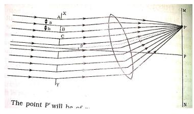
Let *a* is the width of transparent part (slit) and *b* is width of opaque part (line drawn) then (a + b) is called grating element. If there *N* lines per meter in grating then  $(a + b) = \frac{1}{N}$
