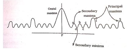
Suppose the angle of diffraction is increased by an amount  $d\theta$ , such the path difference between the secondary waves from *A* to *C* increased by  $\frac{\lambda}{N}$
